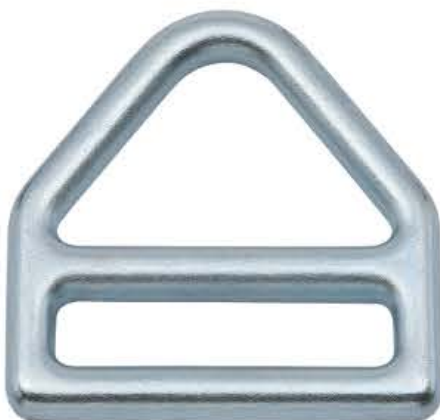
YID022 MATERIAL High Tensile Steel Alloy MINIMUM BREAKING STRENGTH 25kN/5620LBS WEIGHT 56 g FINISH Nickel-chromed,White/Yellow Zinc SPECIFICATION > Webbing: 44 mm > Width: 58 mm > Length: 55 mm
