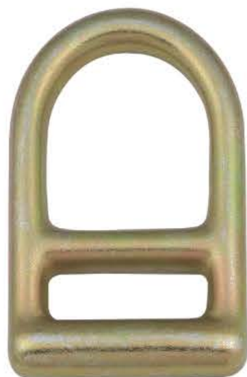
YID007 MATERIAL High Tensile Steel Alloy MINIMUM BREAKING STRENGTH 25kN/5620LBS WEIGHT 86 g FINISH Nickel-chromed,White/Yellow Zinc SPECIFICATION > Webbing: 32 mm > Width: 47 mm > Length: 72 mm
