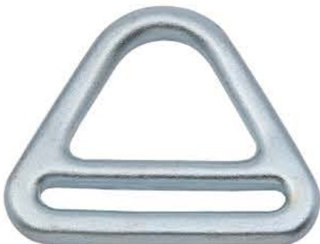
YID021 MATERIAL High Tensile Steel Alloy MINIMUM BREAKING STRENGTH 25kN/5620LBS WEIGHT 41 g FINISH Nickel-chromed,White/Yellow Zinc SPECIFICATION > Webbing: 45 mm > Width: 59 mm > Length: 45 mm
