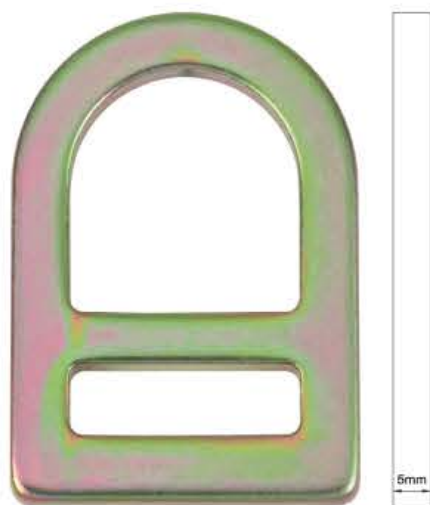
YID026 MATERIAL High Tensile Steel Alloy MINIMUM BREAKING STRENGTH 22kN/5000LBS WEIGHT 76 g FINISH Nickel-chromed,White/Yellow Zinc SPECIFICATION > Webbing: 31 mm > Width: 47 mm > Length: 66 mm
